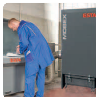
The MOBEX-dust extractors can also be used in combination with an ESTA Extraction table.
