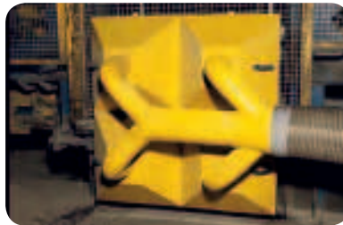
Large surface extraction hood in the concrete industry
