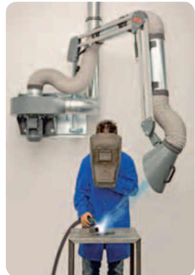
Extraction unit RG-200 with 3.0m extraction arm
