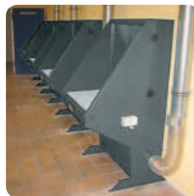
Multiple ESTA welding tables connected to an extraction and filtration system
