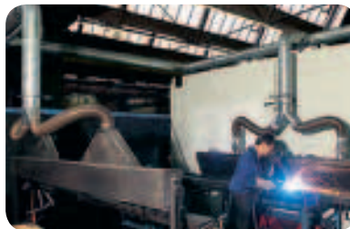
Slotted extraction hoods in the automotive industry
