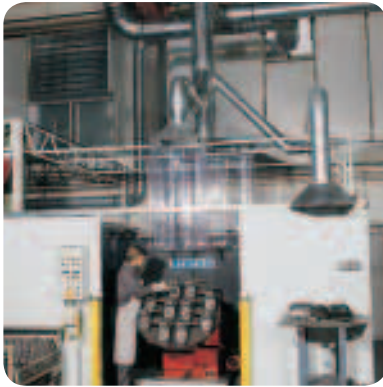
Extraction at a robotic welding station
