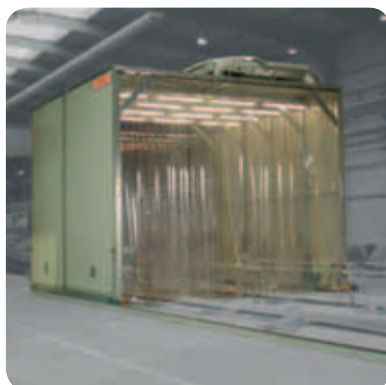
Mobile sanding station
