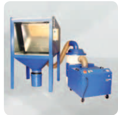
DUSTOMAT 160-S in OEM-version for dust extraction on a manual flocking workstation
