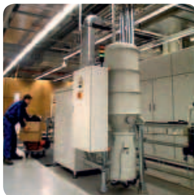
Cyclonic filter FZ-1003 with 100Litre collection container
