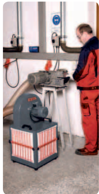
ESTA 100 connected to a belt sanding machine
