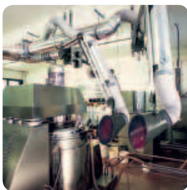
Source capture with two extraction arms
