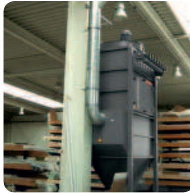
Extraction system DUSTMAC XS-17 with fan mounted on top
