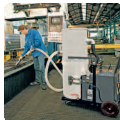
Removal of brass shavings and coolants at a CNC milling station
