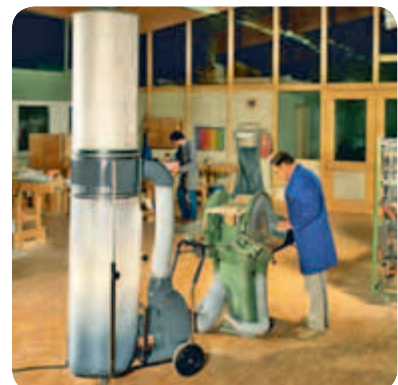
Mobile extraction unit with cartridge filter
