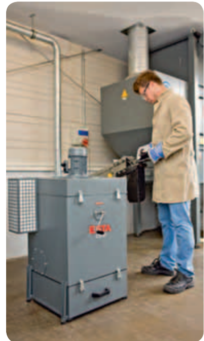
OM-8 connected to a belt sanding machine
